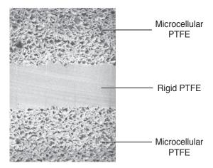
Cross-sectional view under electron microscope All layers manufactured using proprietary GYLON® process—thermally fused layers, without the use of adhesives
