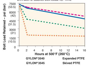
High bolt load retention of GYLON® 3540 and 3545, especially at high temperatures, indicates gasket is less likely to incur gross leakage (blowout).
