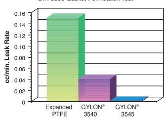
Note the dramatically reduced leakage of GYLON® 3540 and 3545. Average of three tests, using 580 psig nitrogen with 4,640 psi gasket load according to DIN 3535 requirements. All samples 1/16" (1.6 mm) thick.
