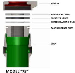
**SPECIFICATIONS Bottom Thread** 8-5/8" O.D. 8rd\* **Bottom Connection** Male **Working Pressure** 1500 PSI 3000 PSI **Test Pressure** Max. Slip Load (2:1 SF) 100,000 lbs. 9-5/8" API Modified\*\* **Cap Thread Cap Material Ductile Iron** 4-1/2", 5-1/2" **Inner String** Suspension Slip or Mandrel **Side Outlet** 2" LP **Minimum Bore** 8.000" **Body Material** Carbon Steel 13-3/4" Height Weight 161 lbs.
